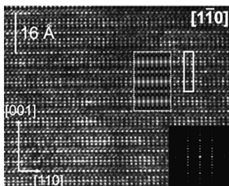
Figure 6. Theoretical ( f = -35 nm, t = 12 nm, dashed outline) and experimental [1\bar{1}0] zone HRTEM image of \text{Ni}_3\text{GaTe}_2 . The corresponding Fourier transform is shown as an inset. A solid line outlines the unit cell.
